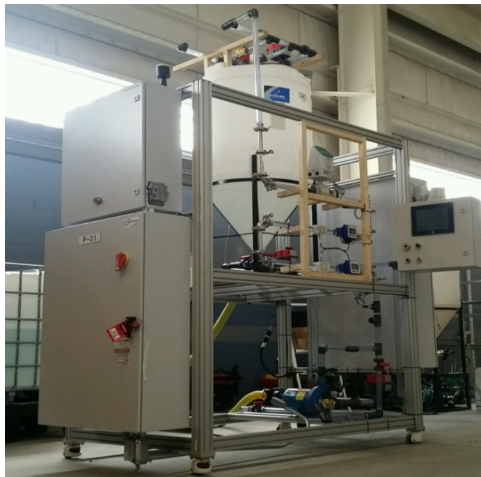
Figure 3. Automation Flow Trainer
