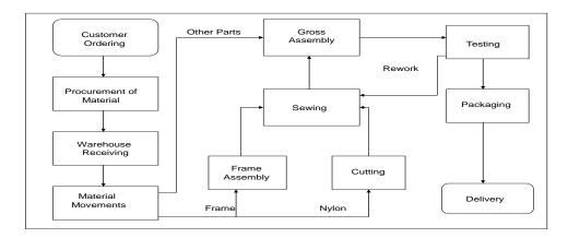
Figure 1 The Manufacturing Process of China Umbrella Factory Limited
